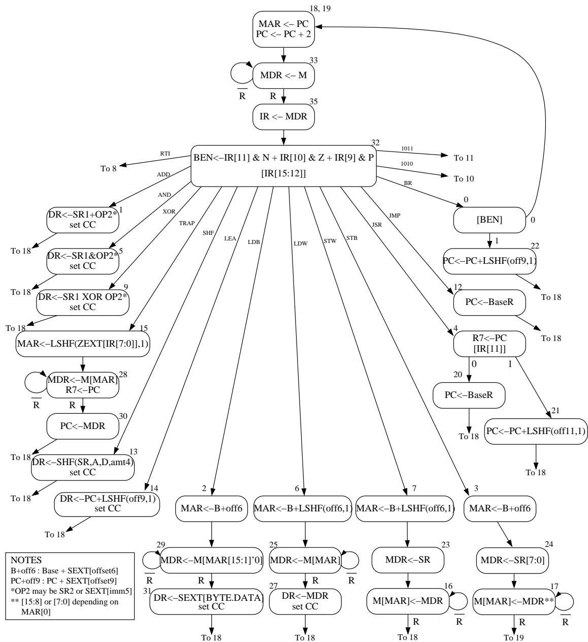
Figure C.2: A state machine for the LC-3b
