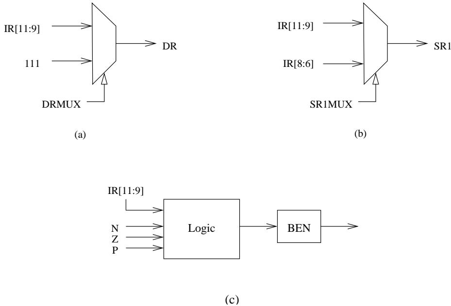
Figure C.6: Additional logic required to provide control signals
