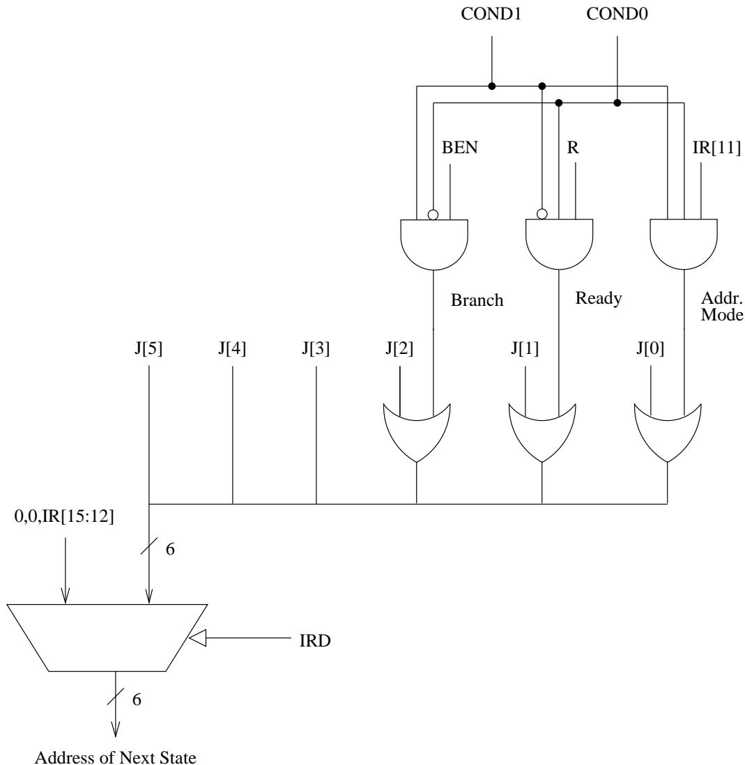
Figure C.5: The microsequencer of the LC-3b base machine
