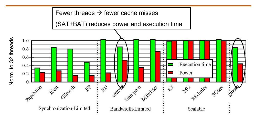
On average, (SAT+BAT) reduces the execution time by 17% and power by 59%
